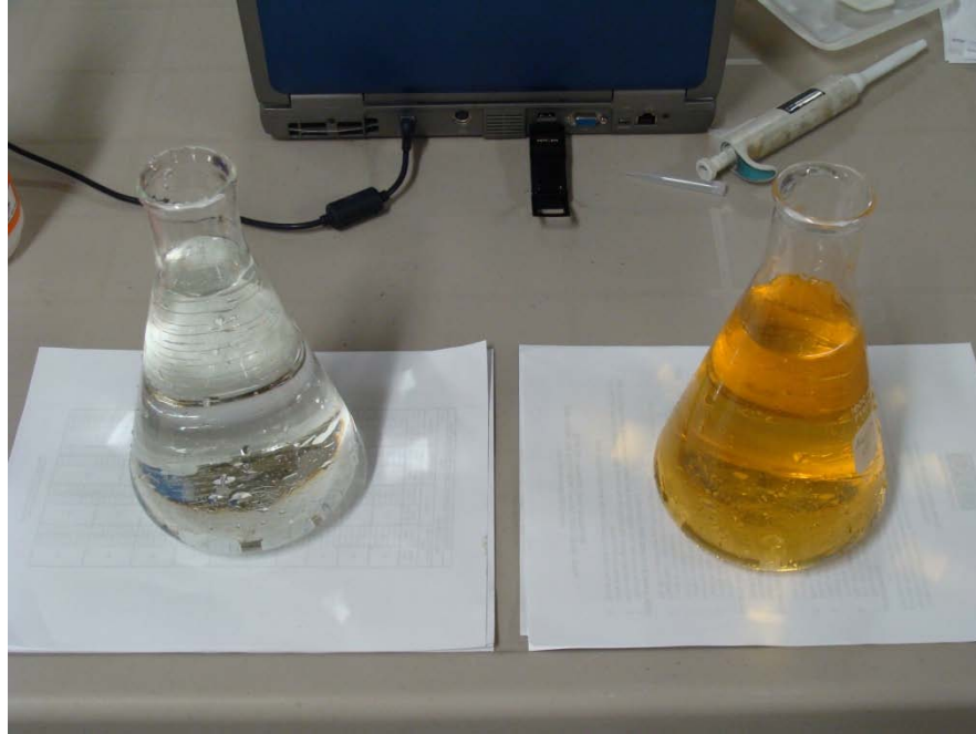
Figure 3. Impact of oxidation by chlorine dioxide on dissolved Mn in Canton raw water. Applied chlorine dioxide dose = 1.5 mg/L, pH = 7.4. Raw water Mn concentration not known.
